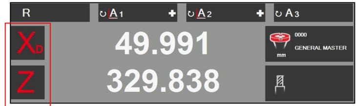
Clicking on X and Z opens a pop-up window in which the different "axis measurement modes" can be selected.
