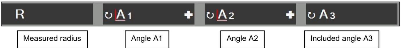
Click the '+' sign to open a window in which the angle calculation base and measurement angle direction can be modified.
