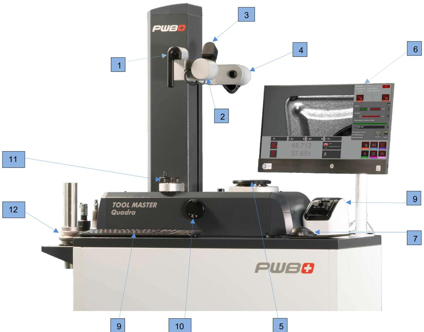
1. Handle to lock/unlock and move both axes
